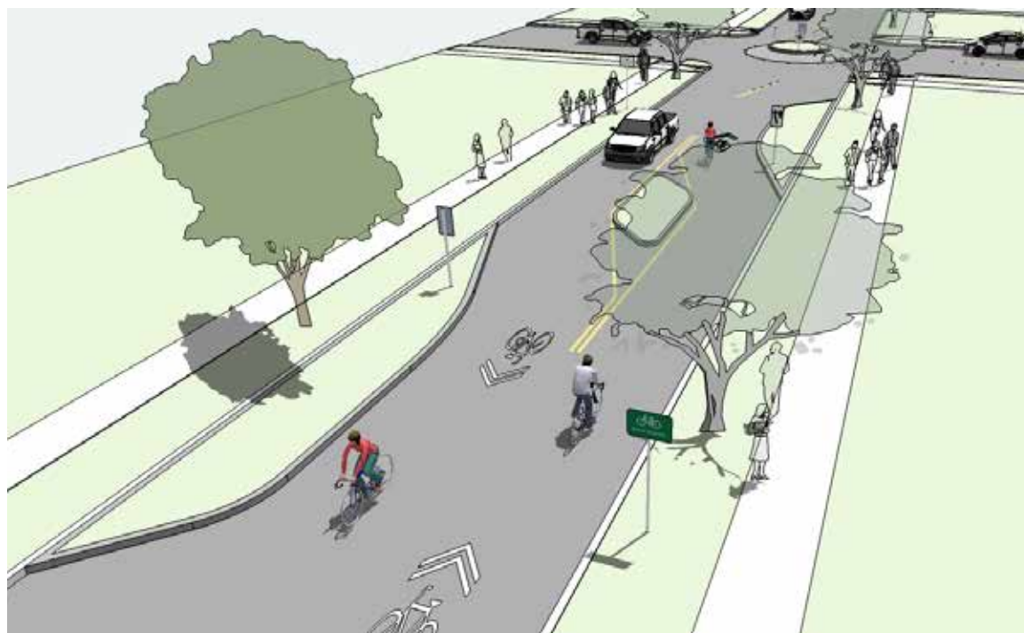
Bicycle boulevard diagram using curb extensions for speed control
