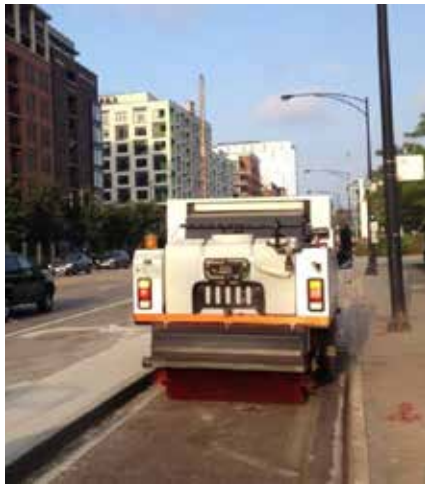
Maintenance Considerations: Seven and a half foot clear zone in Chicago, IL. Source: Chicago Department of Transportation
