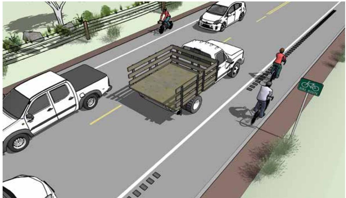
Diagram of paved shoulder use as a bike network component.
