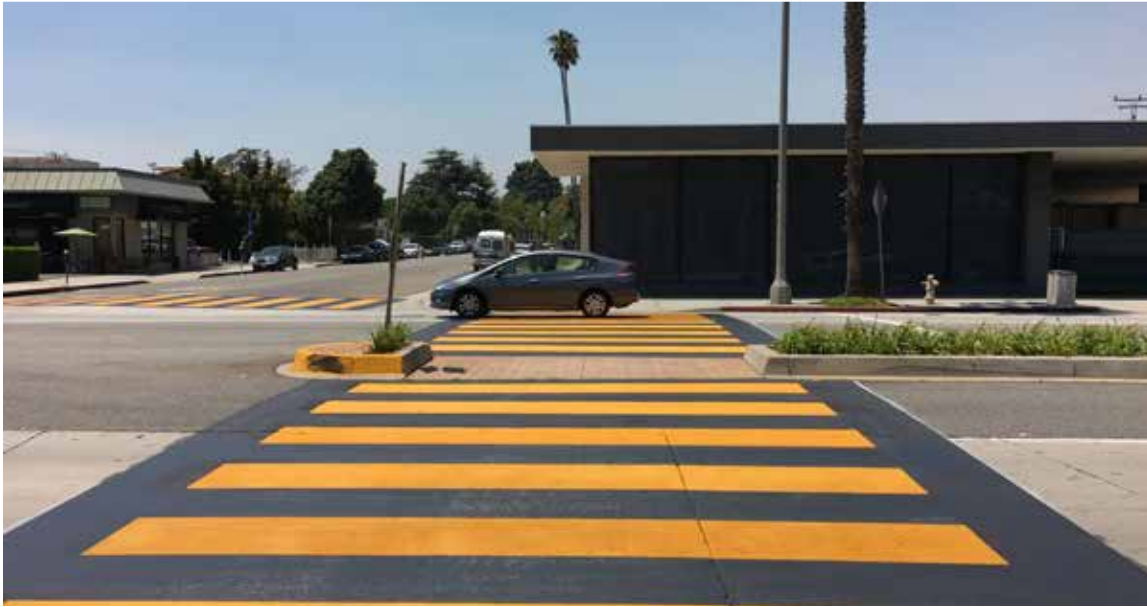
Figure 6.7: Intersection Concepts, High Visibility Crosswalks
