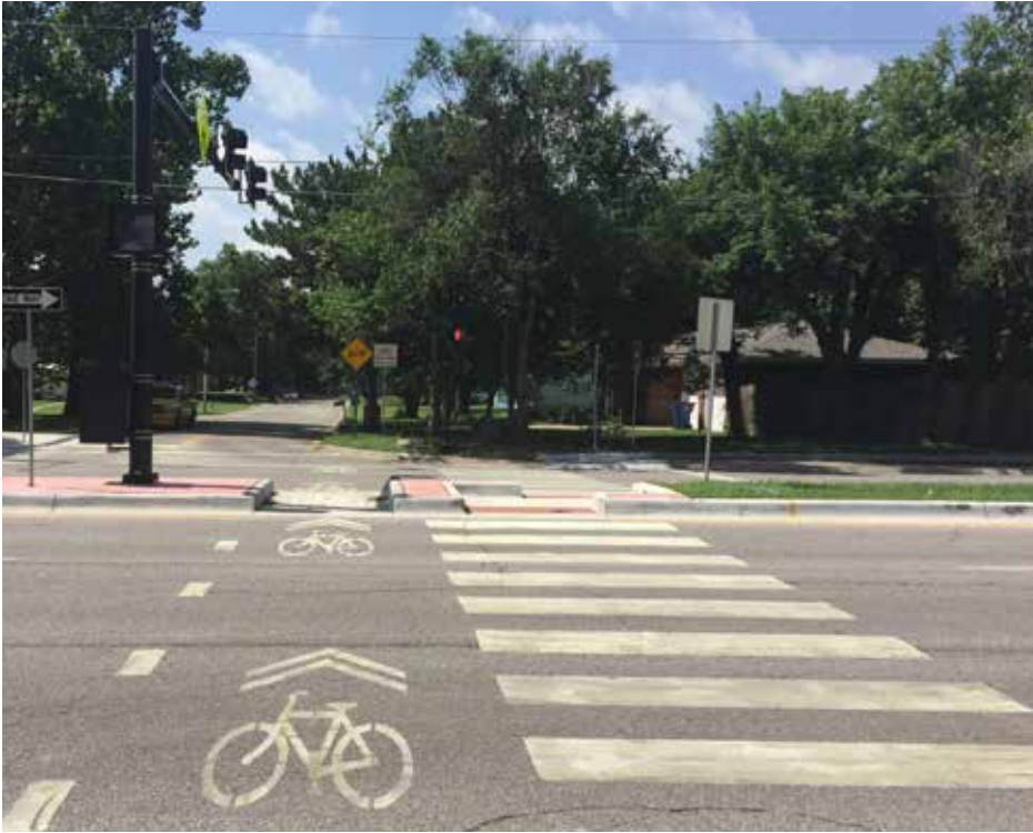
Clockwise from left: HAWK signal and crosswalks on Woodchuck Bicycle Boulevard in Wichita, KS; flashing beacon in Wauwatosa, WI; advance warning and beacon on Prairie Sunset Trail in Goddard, KS
