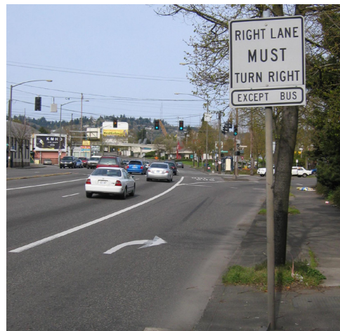
Targeted queue bypasses improve service reliability and help buses maintain schedule adherence.
